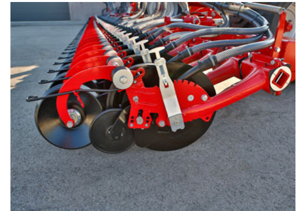
Perfect fixation of the seed due to rubber catching roller
