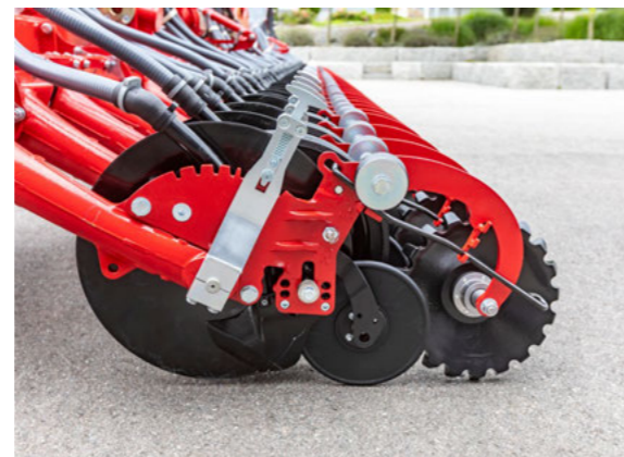
Steel star roller produces fine soil and closes the seed furrow
