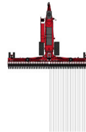
Saving seed due to half-width shut-off
