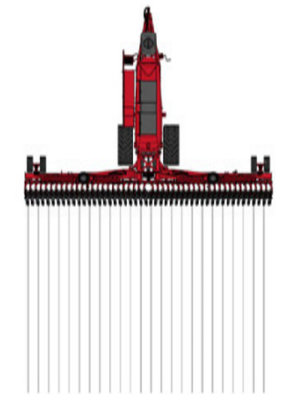
Selective hosing - doubling the row spacing from 25 cm to 50 cm
