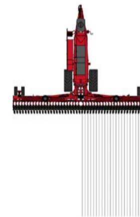
Saving seed due to half-width shut-off
