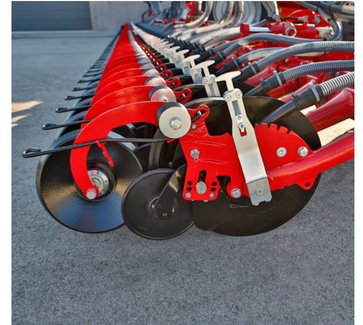
Perfect fixation of the seed due to rubber catching roller
