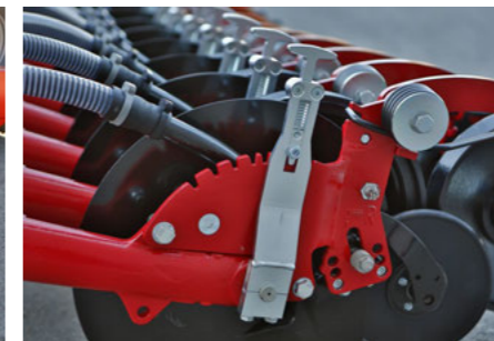
Finely graduated individual depth adjustment without tools
