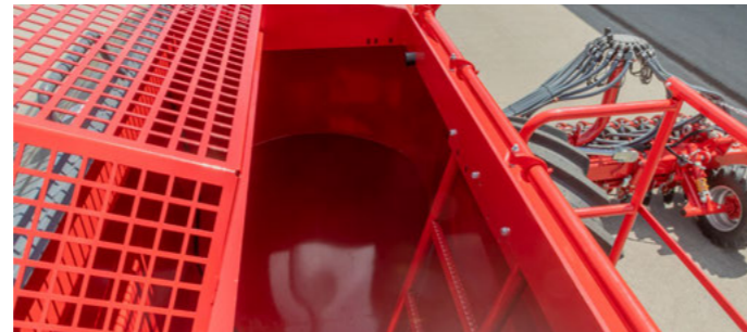
Hinged screens to prevent contaminations in the hopper
