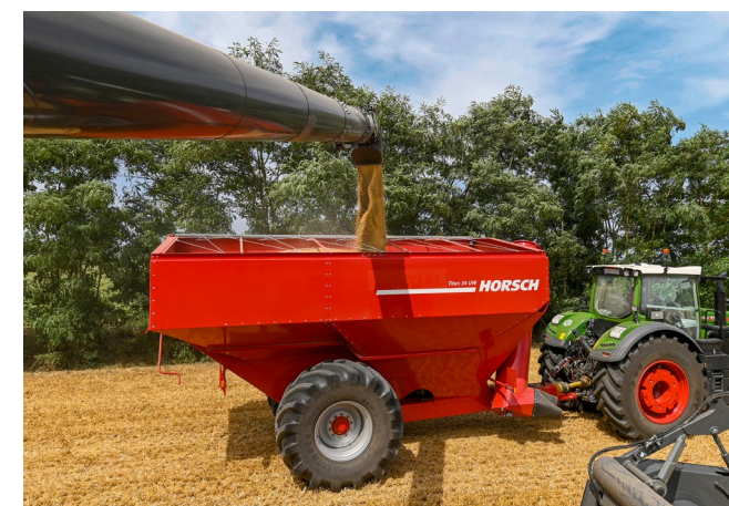
Flexible use due to 4.6 m transfer height and excellent visibility
