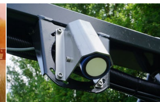
Extension by another pair of ultrasonic sensors
