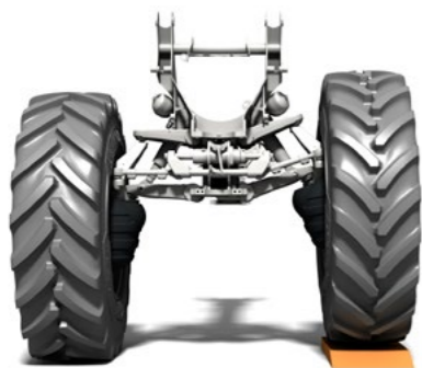
Automatic level regulation: every tyre is spring-loaded and balanced in an hydro-pneumatic way.
