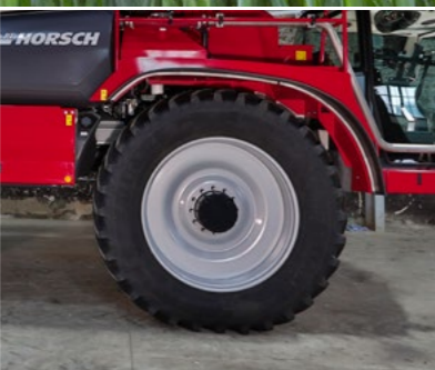
Large tyres with a diameter of up to 2.18 m
