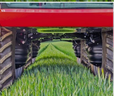
Underbody cover and fairing of the wheel motors protect the population
