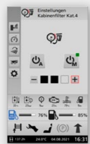
Adjustment options for cabin filter Cat. IV: automatic or manual mode with adjustment to the required intensity
