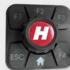
Simple navigation in the vehicle display with a push-turn control knob
