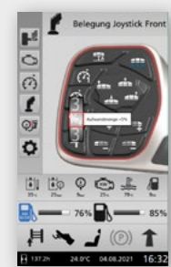
The function of softkeys on the joystick of the ErgoControl can easily be selected via the vehicle display
