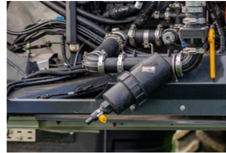
Second pressure filter in the middle frame of the boom
