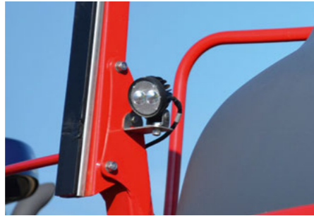
Boom apron lighting
