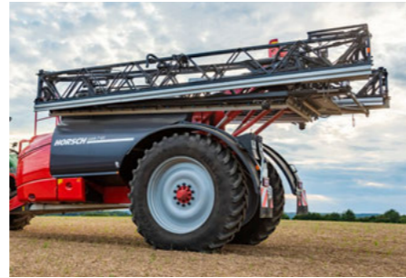
Tyres with Ø 2.07 m for maximum clearance and contact area
