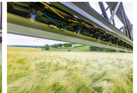
Pneumatic nozzle and section control e.g. 3D application
