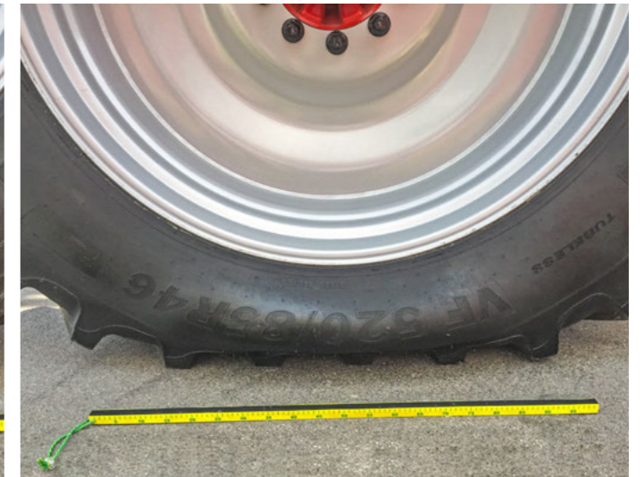
ATP Control – increased contact area at 1.0 bar tyre pressure
