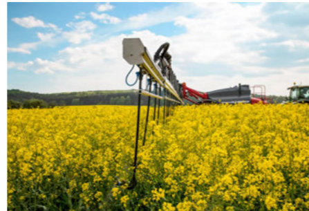
Systems for under leaf spraying, e.g. droplegs
