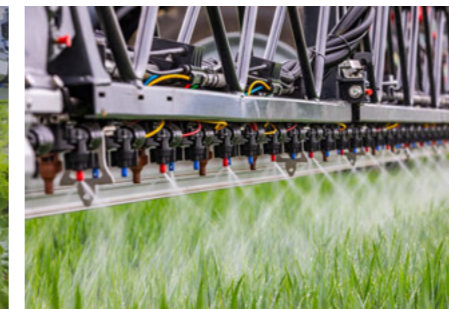
25 cm nozzle layout: more nozzles more possibilities e.g. 3D application
