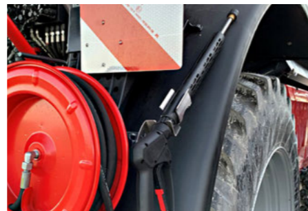
Hydraulically driven high-pressure cleaner
