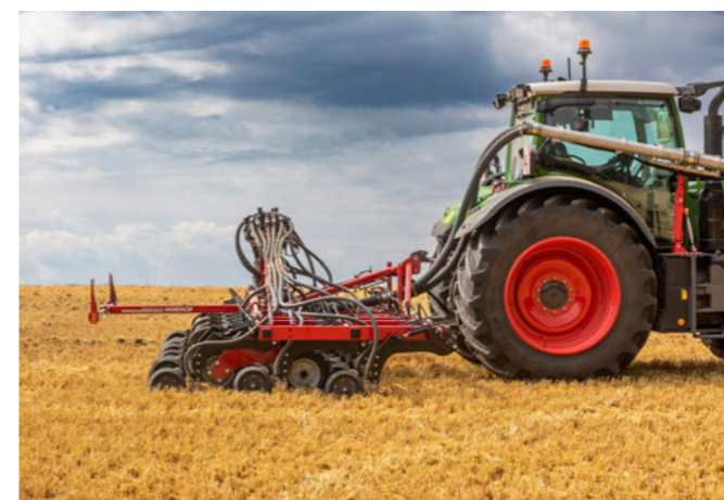
3-bar design for maximum clearance
