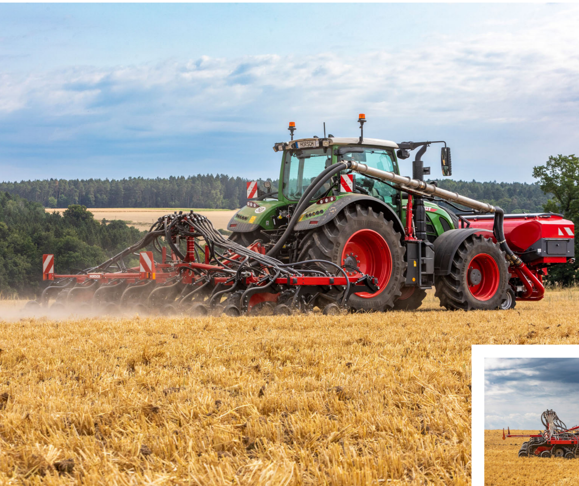
3-bar design for maximum clearance
