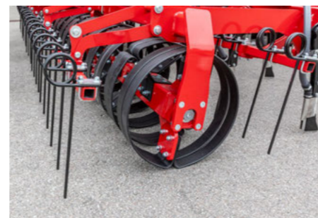
Harrow in front of and behind the packer for a perfect covering of the seed
