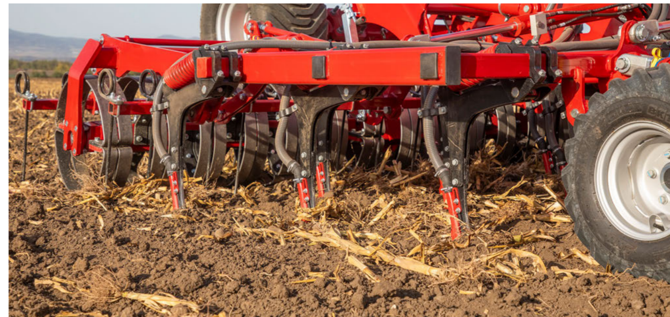
Residue-free seed furrow due to clearing effect of the tine
