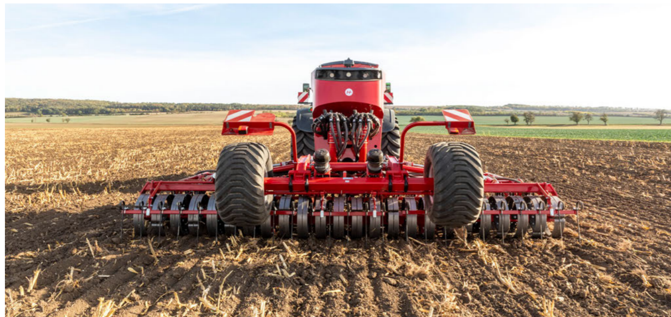
Even consolidation due to packer
