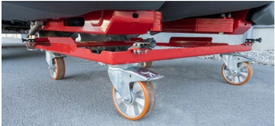
The robust shunting roller waggon facilitates the handling of the front tank
