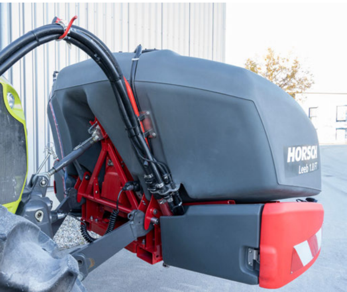
Leeb FT Pro with hose holder and hose routing
