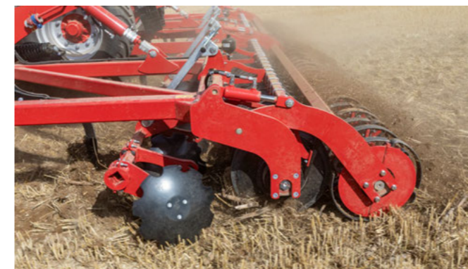
Hydraulically pre-tensioned packer
