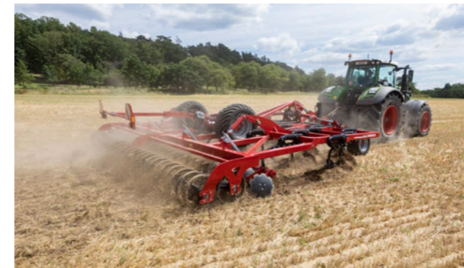
Rigid packer frame with double RollPack packer
