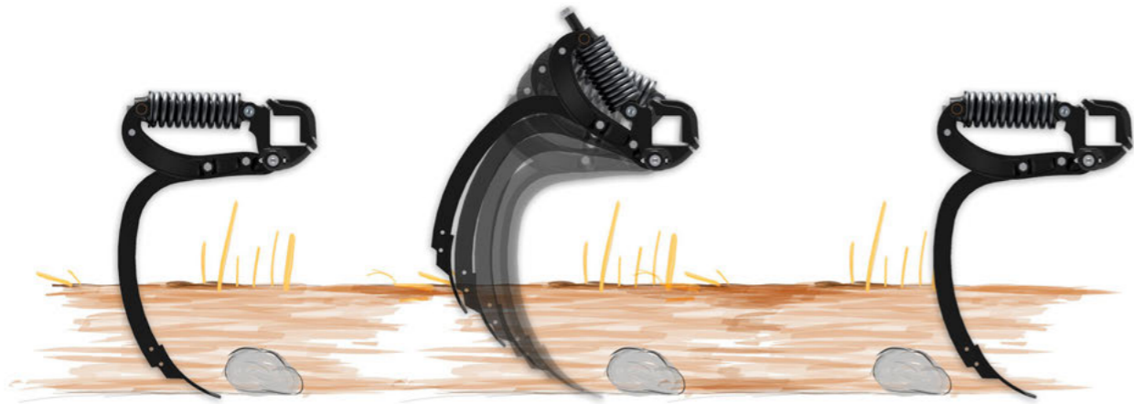
TerraGrip III – release effect
