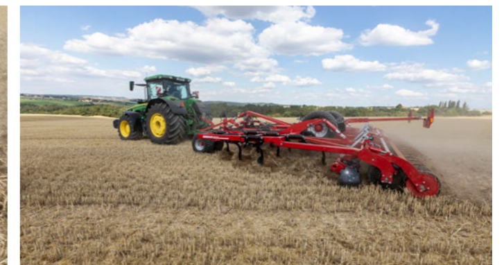
Steelflex packer with hydraulically pre-tensioned RingFlex
