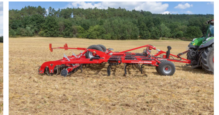
Rigid packer frame with double packer
