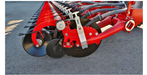
Perfect fixation of the seed due to rubber catching roller
