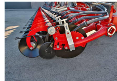
SingleDisc – perfect soil following due to depth control wheel
