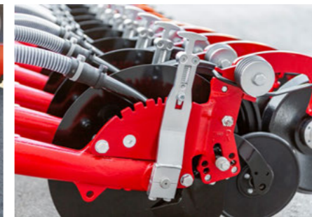
Finely graduated individual depth adjustment without tools
