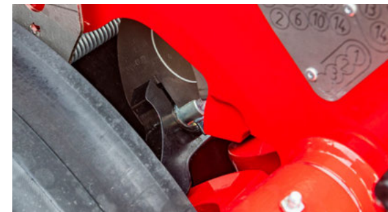
The Piezo sensor in detail
