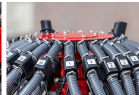
Spelt pneumatics for husk-bearing seeds
