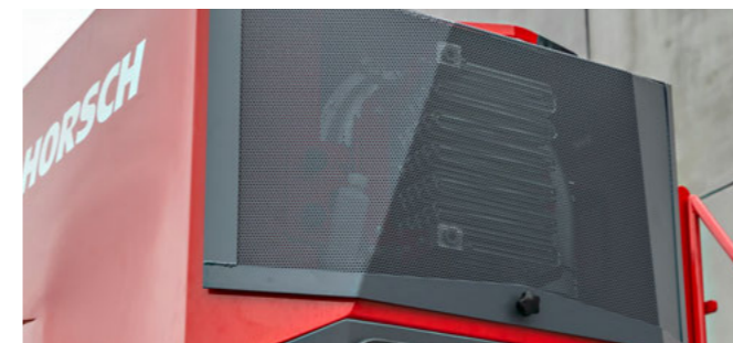
Oil cooling on the hydraulic fan – heats the air flow in the pneumatic system
