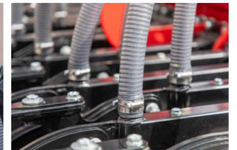
Optimised pneumatic hosing and chamfered seed tubes
