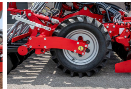
Low horsepower requirement due to large tyre diameter and no scrapers required
