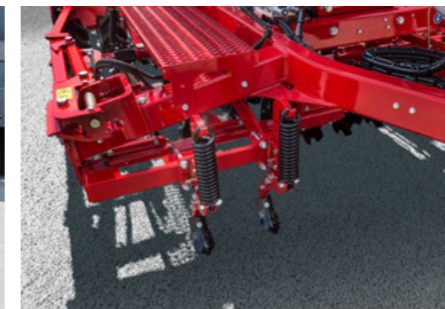
Spring-loaded track eradicator tines loosen soil compactions in the tractor track
