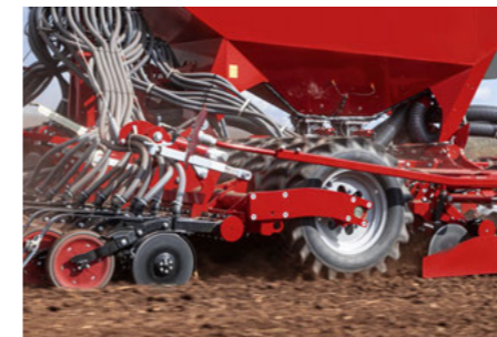
Efficient consolidation below the seed horizon for better water distribution towards the seeds
