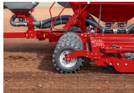
Lowest possible track depths of the tractor in the seedbed
