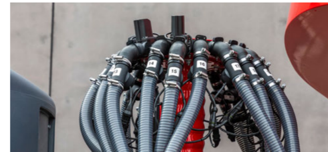
Fertiliser and seed flow monitoring – for a permanent monitoring of the seed and fertiliser hoses
