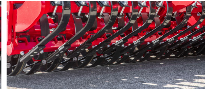
Infinitely variable, hydraulic working aggressiveness adjustment
