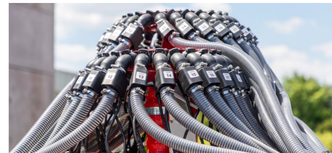
Fertiliser and seed flow control – for a permanent monitoring of the seed and fertiliser hoses
