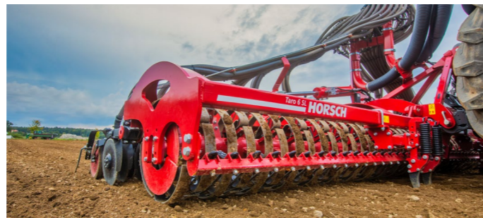
RollFlex packer: deep consolidation, crushing of clods
