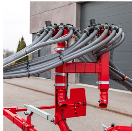
It is possible to switch off a distribution tower and thus every second seed row
