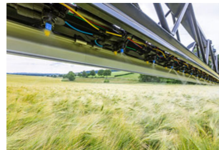
Pneumatic nozzle and section control
