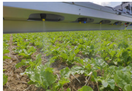
Band spraying is also no problem for a 25 cm spacing
