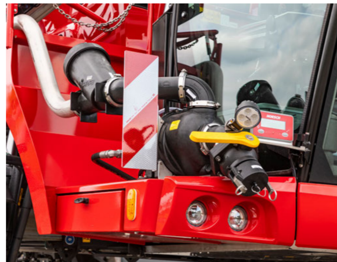
PowerFill filling pump with 1000 l/min output – 3" Camlock filling connection front right
