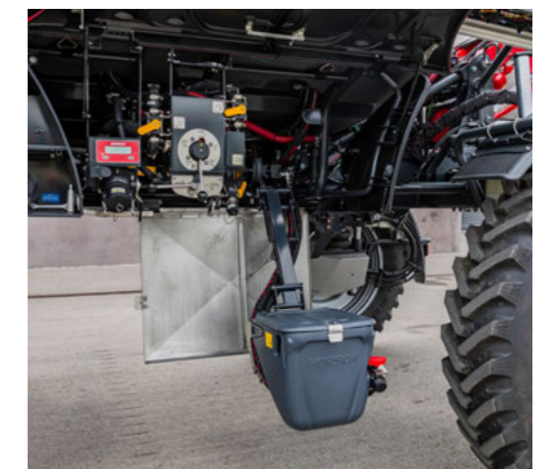
Water system CCS
