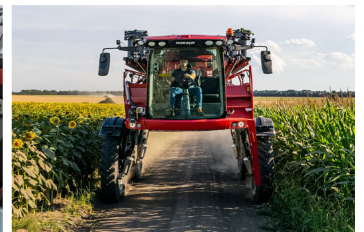
Variable clearance from 1.60 m to 2.40 m
