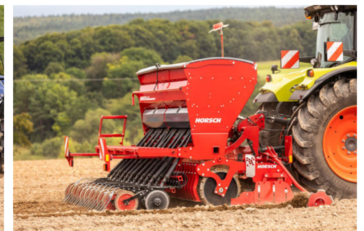
Versa 3 KR – 1 500 l hopper capacity
