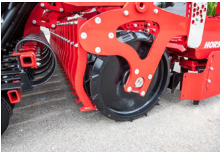
Trapeze ring packer 60 cm diameter
