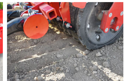
FarmFlex packer Strip consolidation reduces encrusting
