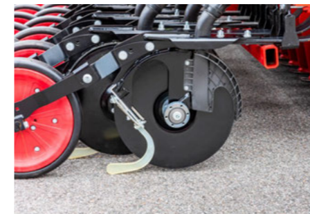
Fall tube position in front of the mounting and moving inside scraper prevent blockage of the coulters in wet sowing conditions
