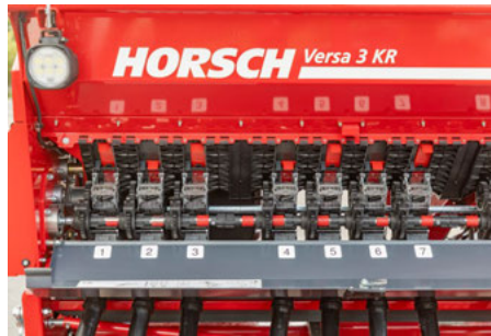
SmartClip metering system – tramline control
