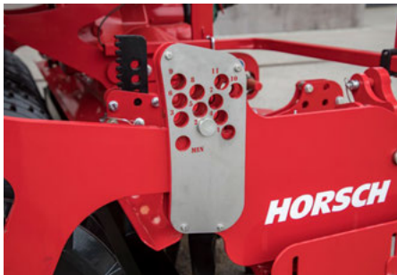
Adjustment of working depth without tools via the hole pattern between Kredo and packer
