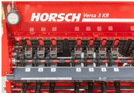
SmartClip metering system – tramline control
