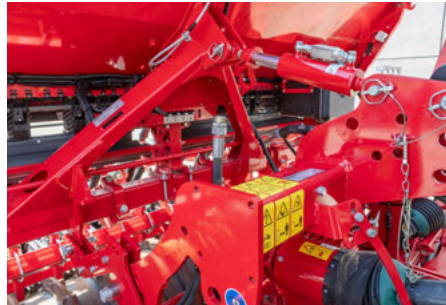
Hydraulic upper link between rotary harrow and Versa KR
