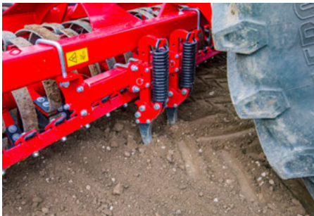
Spring-loaded track-eradicator tines
