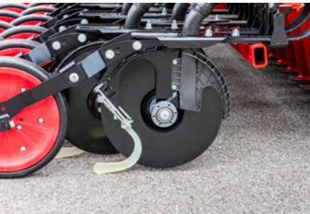
Fall tube position in front of the mounting and moving inside scraper prevent blockage of the coulers in wet sowing conditions
