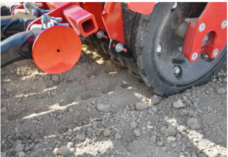
FarmFlex packer Strip consolidation reduces encrusting
