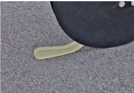
The HORSCH Uniformer – TurboDisc seed couler ensures a precise fixing of the seed
