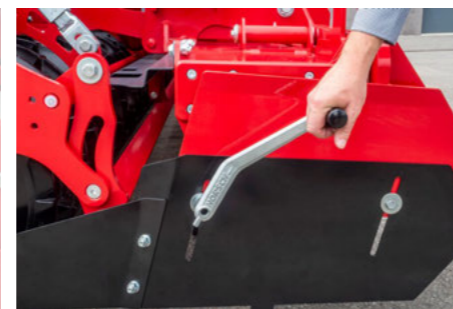
Adjustment of the side panels with the universal key
