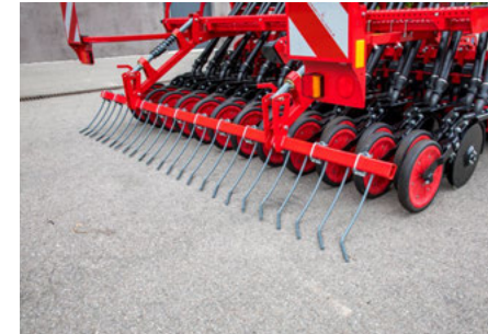
Heavy harrow: the ideal solution for late sowing in wet conditions
