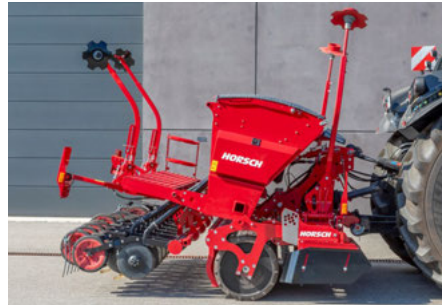
Seed coulters can be lifted to use the rotary harrow solo on the headlands or in field corners
