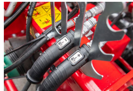
Clearly marked hydraulic connections
