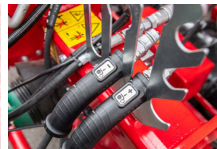
Clearly marked hydraulic connections
