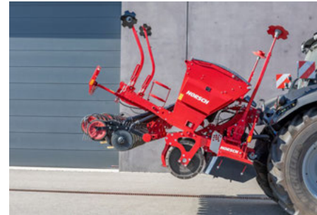
The hydraulic cylinder can be retracted for more clearance for road transport
