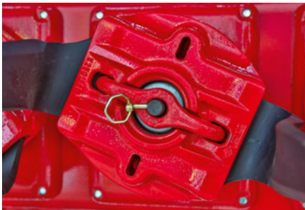
Tines can be changed without any tools
