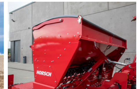
1 500 l hopper attachment: less filling stops due to increased hopper capacity
