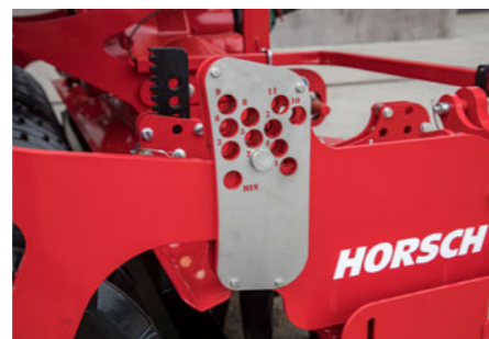
Working depth adjustment Versa SL R via locking pin on a clearly visible stainless steel scale
