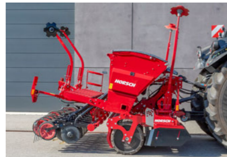
Preparatory work with the rotary harrow on the headlands or in field corners with lifted seed coulters
