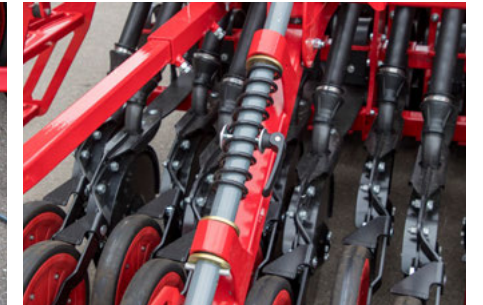
Easy pressure adjustment of the heavy harrow
