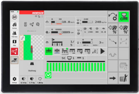
By displaying up to 3 widgets in addition to the main working screen, the user can keep track of several applications at the same time
