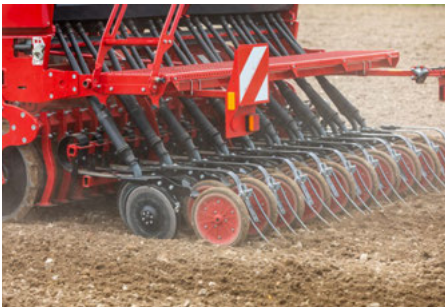
DuoDisc seed coulers with straight harrow
