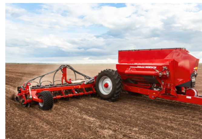
Due to the sliding axle, the wide tyres run between the rows
