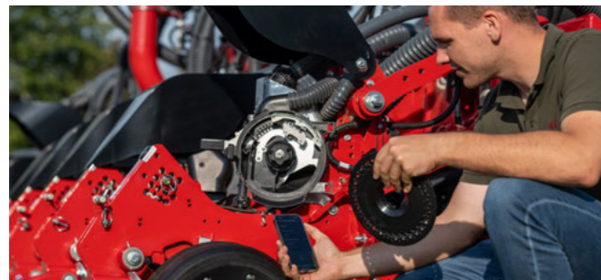
The HORSCH Assist app with the „Metering Disc Selection“ function helps you to select the optimal metering disc for every application.
