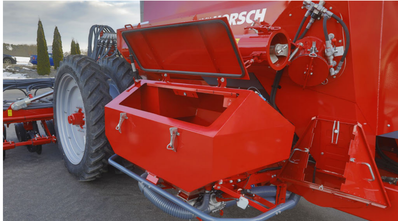
Microgranular unit For filling and to increase the accessibility of the machine, the hopper can be swivelled forward
