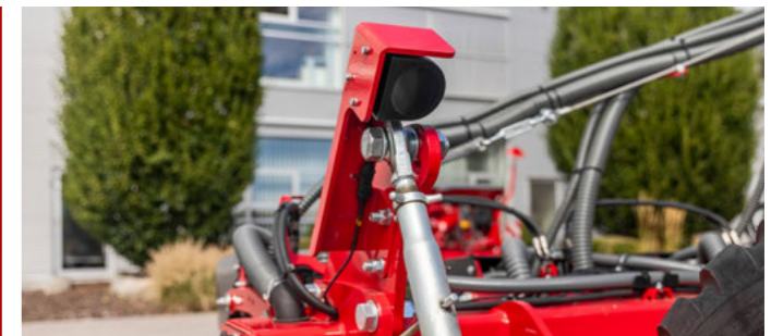
One of the additional radar sensors for ContourFarming
