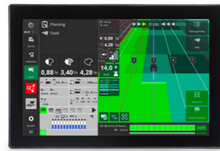
With single grain seeding technology and HORSCH AutoLine, tramlines can be sown completely flexibly and independently of the driving direction supported by GPS.
