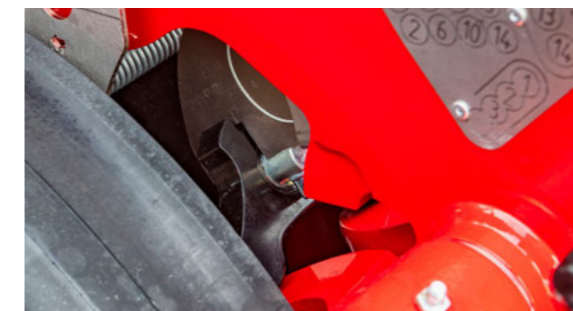
The Piezo sensor in detail
