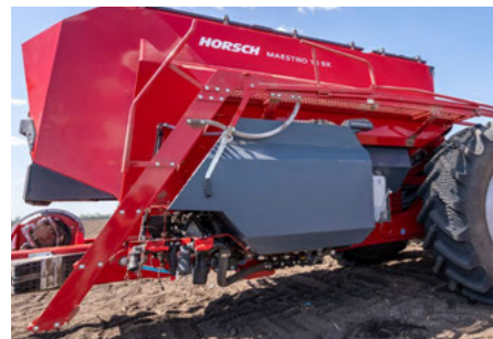
CLT system with 800 l tank capacity
