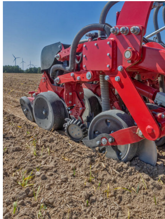
Single disc fertiliser couler
