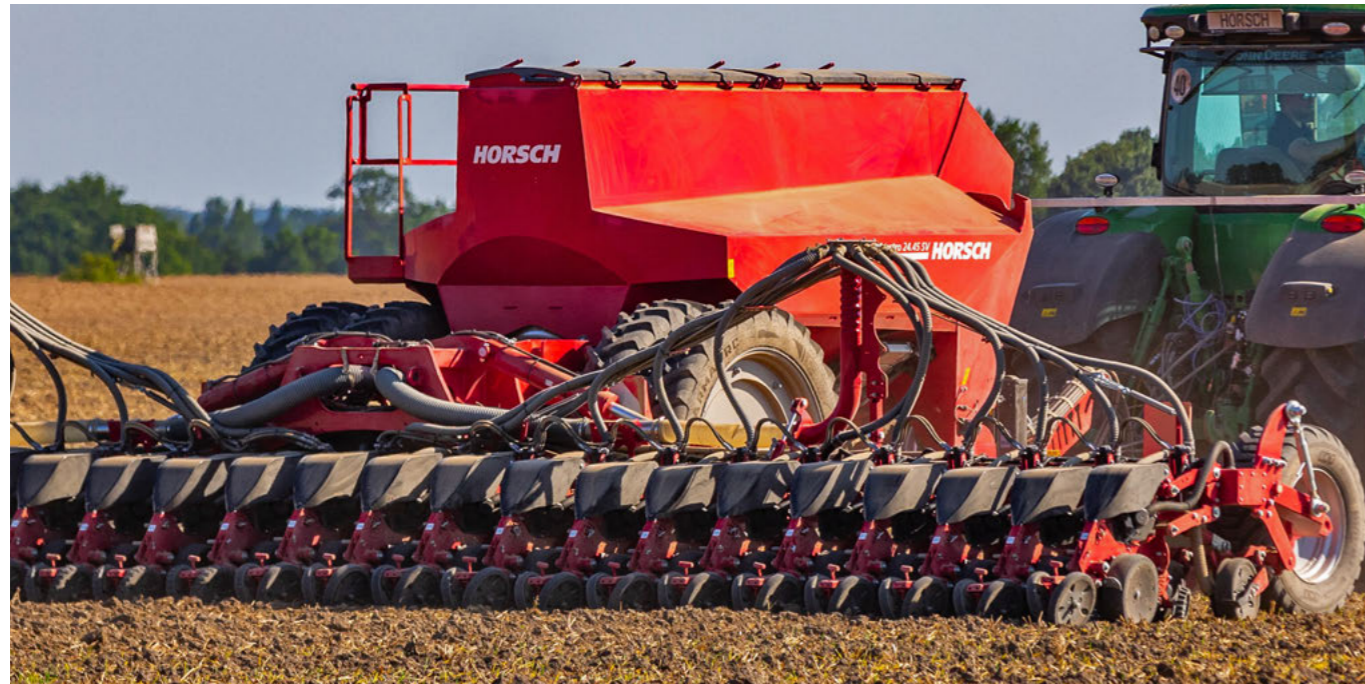
MTS hopper with a capacity of 800 l
