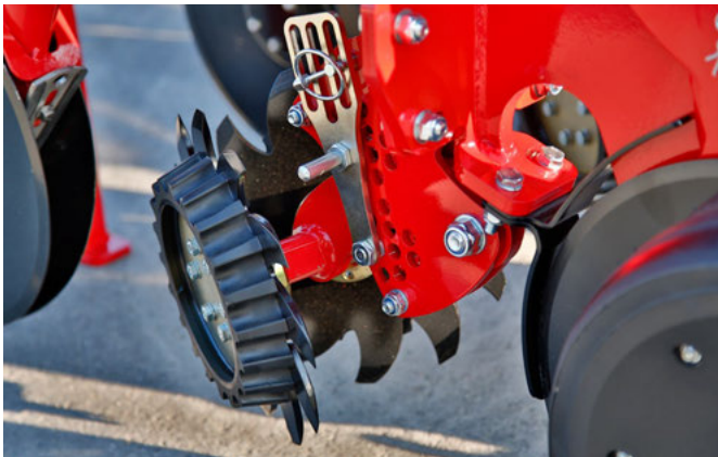
Optional trash wheels, floating with depth control
