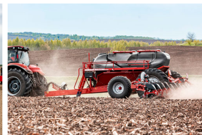
Weight transfer from the seed wagon to the seed bar for a high coulter pressure of up to 350 kg
