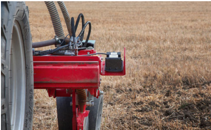
One of the additional radar sensors for ContourFarming
